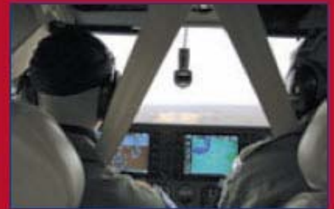
With 129 glass cockpit Cessna 182 Skylanes now in CAP's versatile fleet of 550 aircraft, more CAP aircrews are benefiting from Cessna's state-of-the-art Garmin G1000 flight equipment. The all-glass, jet-like cockpit provides more situational awareness for CAP pilots as well as a collision avoidance system, which helps ensure their safety.
